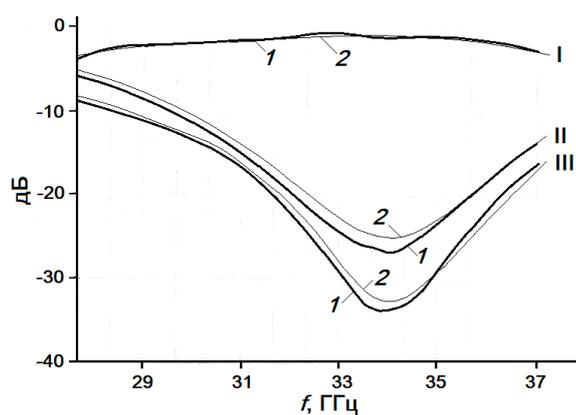
**Figure 2.** Measurements of losses (I) for reflection coefficient (II), and decoupling between arms (III) in the frequency range 28–37 GHz of the Y-circulator with nanocomposites based on opal matrices, the pores of which are filled with Ni<sub>0.5</sub>Zn<sub>0.5</sub>Fe<sub>2</sub>O<sub>4</sub> crystallites (1) and Co<sub>0.5</sub>Zn<sub>0.5</sub>Fe<sub>2</sub>O<sub>4</sub> (2)
