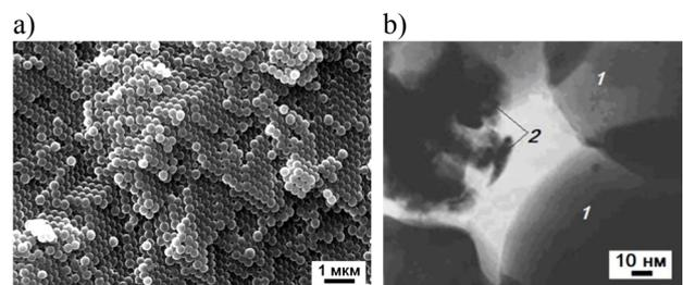
**Figure 1.** a) REM image for the surface of an opal matrix sample; b) TEM image of nanocomposites based on opal matrixes containing crystallites pores:  $\text{Co}_x\text{Zn}_{1-x}\text{Fe}_2\text{O}_4$ ; (1 - spherical particles of  $\text{SiO}_2$ ; 2 - synthesized crystallites)
