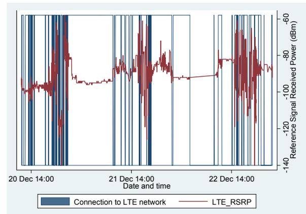
**Figure 1.** Reference Signal Received Power levels (red line) during the connections to LTE network (blue background) over 3-days period, Lyon, France.
