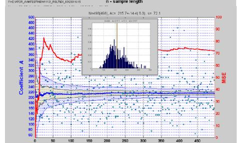
**Figure 1.** Diagrams of the calibration AC values scattering due to random fluctuations of the profiles ZAtt(r) and Z(r) at various noise amplitudes  $\sigma = 0.5, 1, 1.5,$  and 2 dB.
