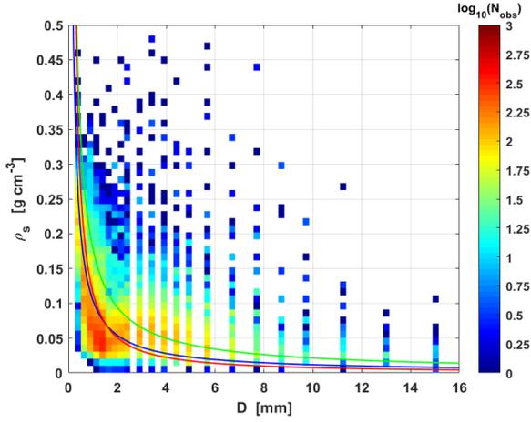
**Figure 2.** Plot of diameter versus density derived from disdrometer measurements. The solid lines indicate the three  $\rho_s$  -  $D$  relations from literature. Green line is from Brandes et al. (2007). Blue line is from Heymysfield et al. (2004). Red line is from Huang et al. (2010).
