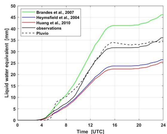
**Figure 7.** Comparison of accumulations at YPO site using  $\rho_s - D$  relations and gauge.
