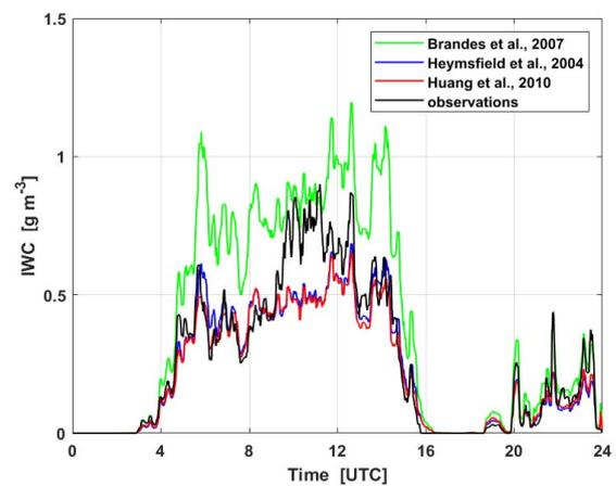
**Figure 6.** IWC using density calculated from disdrometer and three different  $\rho_s - D$  relations.
