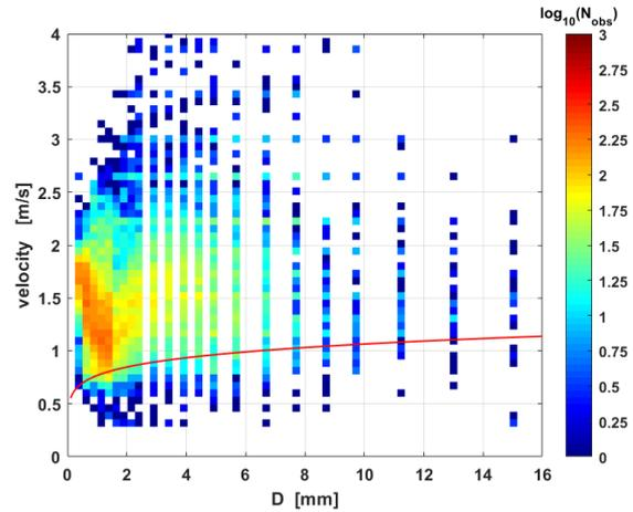
**Figure 1.** Plot of diameter versus velocity for data from 28<sup>th</sup> of February 2018. The red line is empirical terminal velocity of snow from Brandes et al. (2007).
