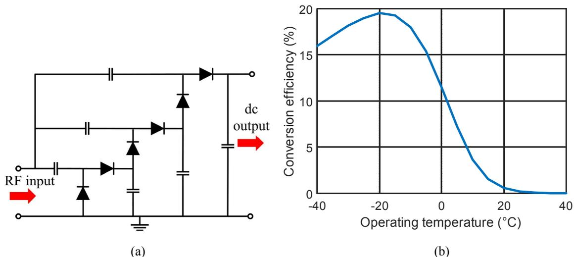
**Figure 1.** (a) Diagram of a 3-stage rectifier based on diodes SMS7630 and (b) its simulation results of conversion efficiency results versus operating temperature in the range of  $-40\text{ }^{\circ}\text{C}$  to  $+40\text{ }^{\circ}\text{C}$ . Matching network influence is de-embedded. Operating frequency is 600 MHz, and load resistance is  $5.8\text{ M}\Omega$ .
