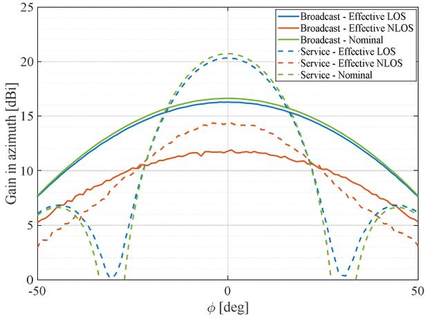
**Figure 3.** Nominal and effective antenna patterns of broadcast and service/traffic beams [8] – magnified view of main lobes
