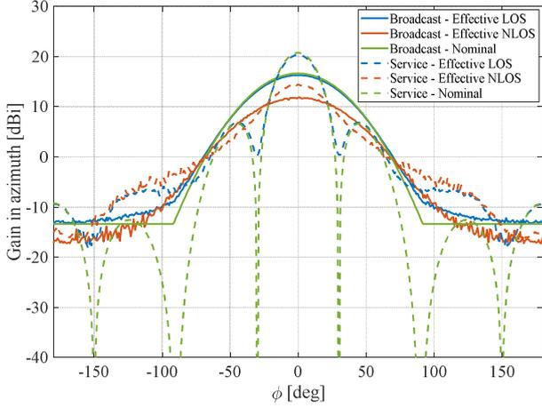
**Figure 2.** Nominal and effective antenna patterns of broadcast/signaling and service/traffic beams [8]
