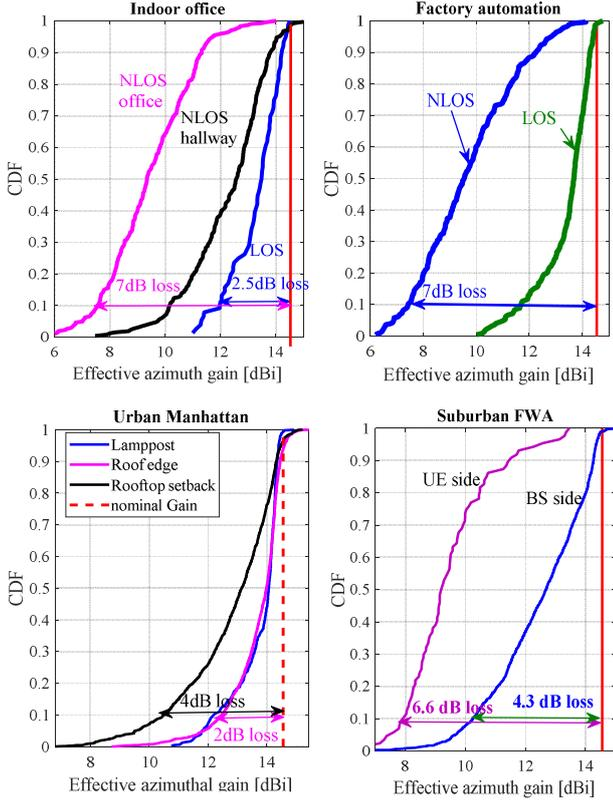
**Figure 1.** CDFs of effective antenna gains measured in indoor office, suburban FWA, factory automation and urban Manhattan environments presented in comparison with nominal antenna gain [4][5][6][7]
