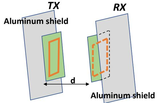
**Figure 9.** Link between transmitter and receiver.
