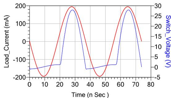
**Figure 11.** Voltage across switch and load current for the realistic link of Fig. 10.
