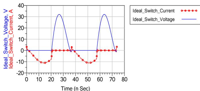
**Figure 5.** Ideal switch waveforms
