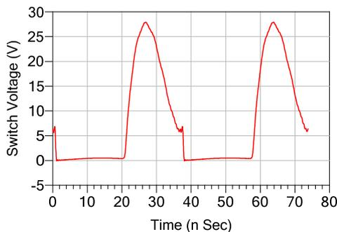
**Figure 8** Switch voltage for the lossy coil
