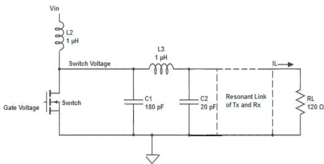
**Figure 1.** Schematic of the WPT link circuit.
