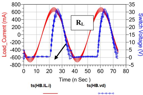
**Figure 7.** Switch voltage for load variation.
