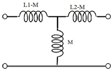
**Figure 2.** Inductive link between Tx and Rx equivalent representation.
