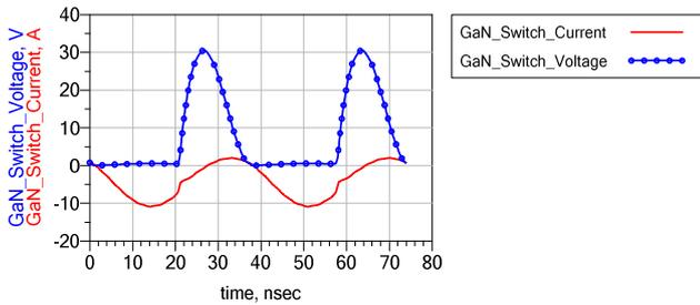
**Figure 6.** GaN Switch waveforms
