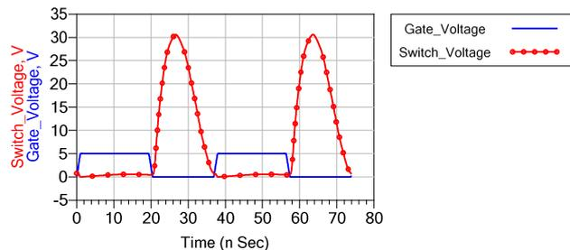
**Figure 3.** Gate and switch voltages for  $k=0.1$ .
