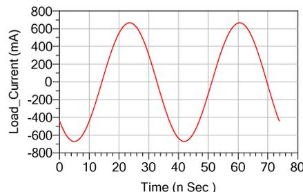
**Figure 4.** Current waveform on the load  $R_L$  for  $k=0.1$
