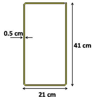
**Figure 10.** Transmitting coil layout.
