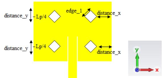
**Figure 2.** Antenna #2 front view.
