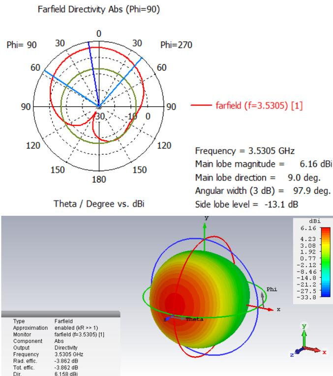
Figure 8. Far field pattern results for the Antenna #4.
