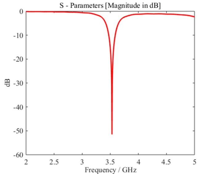
Figure 6.  $S_{11}$  results for the Antenna #3.
