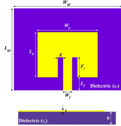
**Figure 1.** Top view and side view of Antenna #1.
