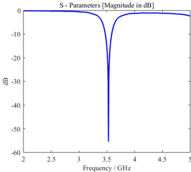
Figure 7.  $S_{11}$  results for the Antenna #4.
