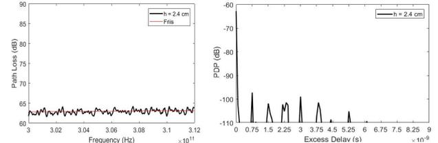
**Figure 4.** (left) Path loss vs. frequency and (right) measured PDP for a smaller size box shown in Fig. 1.
