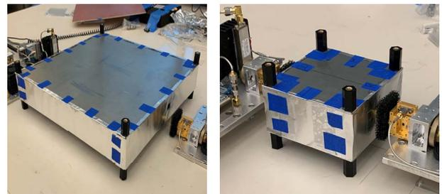
Figure 1. Rectangular metallic cavities used in measurements (left) larger cavity of dimension 30.5 $\times$ 30.5 $\times$ 5cm (right) small cavity 11 $\times$ 11 $\times$ 5cm.
