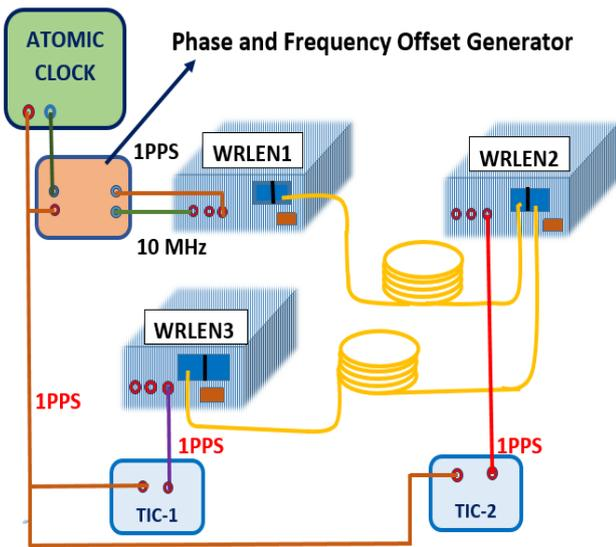
**Figure 1.** Schematic diagram of the experimental setup for testing the stability of the optical fibre link
