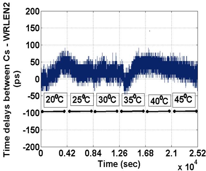
Figure 4. Variation of Time delays for different temperature [mentioned in boxes] of the optical fibre.
