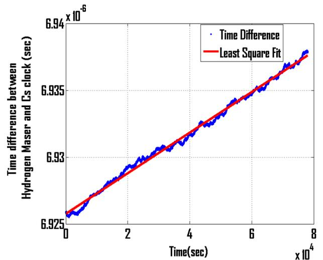
Figure 7. Variation of time difference between the active Hydrogen Maser and the Cs atomic clock. The red line shows the least square fitting of the time variation.
