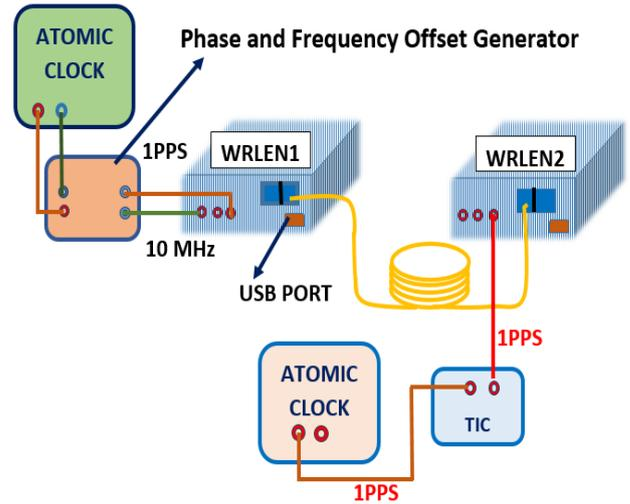
**Figure 2.** Schematic diagram of the experimental setup for comparing stability of atomic clocks.
