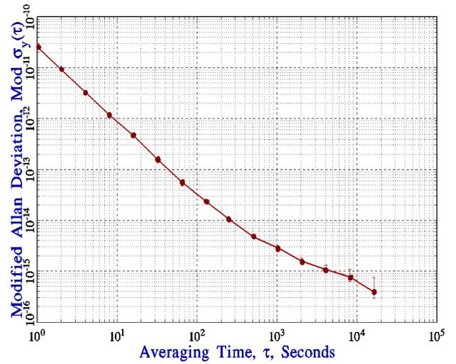
Figure 5. Modified Allan deviation for the time delay data between Cs clock - WRLN2 at ambient temperature ( $19^{\circ}\text{C}$ - $21^{\circ}\text{C}$ ).
