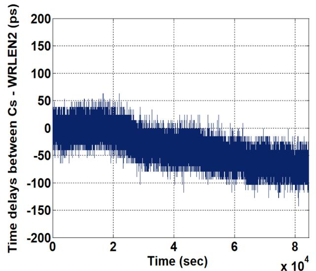
**Figure 3.** Time delays between Cs atomic clock and the WRLN2 after compensating the fixed time offset at ambient temperature ( $19^{\circ}\text{C}$ - $21^{\circ}\text{C}$ ).
