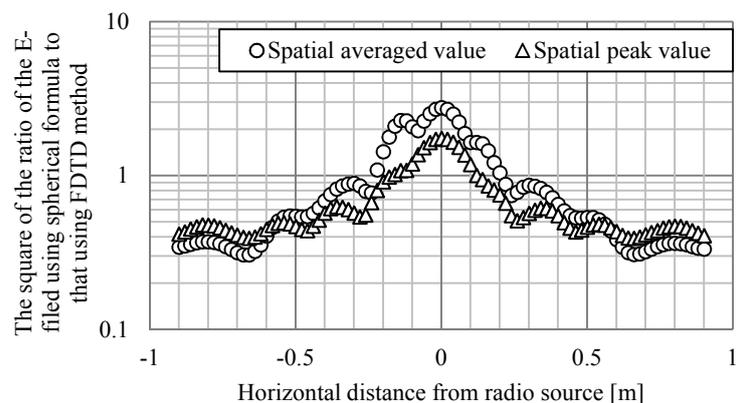
**Figure 2.** A result of the comparisons of the E-field distributions around underground BS using the spherical formula and FDTD method in the direction along the antenna element.
