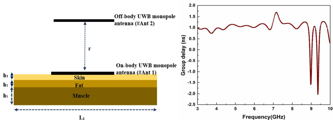
**Figure 1.** (a) Simulation set-up using UWB monopoles for on-body to off-body channel analysis, (b) Simulated group delay characteristics for the setup in Fig. 1(a).
