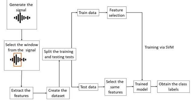
Figure 1. Interference detection process.
