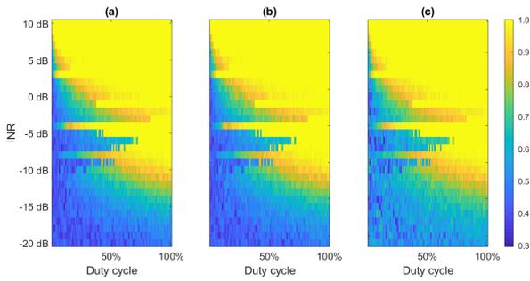
**Figure 2.** Accuracy (a), precision (b) and recall (c) as a function of RFI strength and duty cycle.
