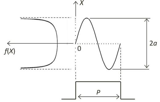
**Figure 2.** Transformation from uniform to U-shaped PDF.
