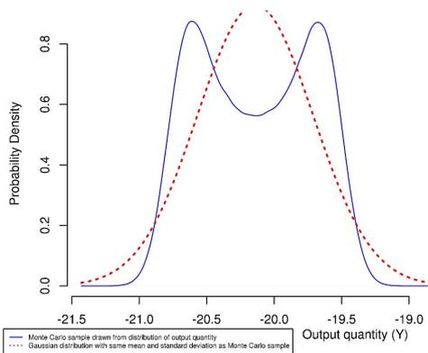
**Figure 3.** PDF of the measured power as obtained through NIST Uncertainty Machine.
