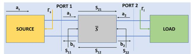
**Figure 1.** Sketch of the connection between a source and a load through a two-port network represented by its scattering matrix  $\bar{\bar{S}}$ .
