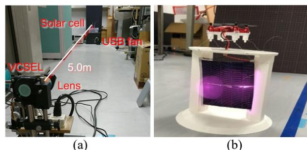
**Figure 2.** OWPT demonstration. (a) 5m-long distance OWPT, (b) flying of micro-drone.
