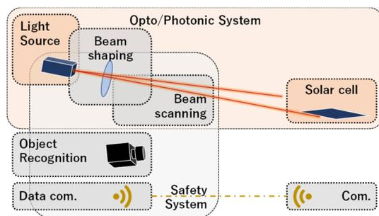
**Figure 1.** Schematic configuration of OWPT system.
