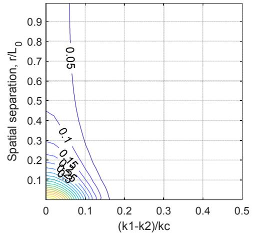
**Figure 3.** Contour plot of the absolute value of the coherence function in the domain  $(k_d/k_c, r/L_0)$ .  $f_c = 400$  MHz,  $L_0 = 10$  km,  $\sigma_N^2 = 0.1$
