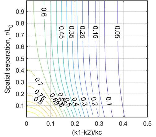
**Figure 2.** Contour plot of the absolute value of the coherence function in the domain  $(k_d/k_c, r/L_0)$ .  $f_c = 1$  GHz,  $L_0 = 10$  km,  $\sigma_N^2 = 0.1$
