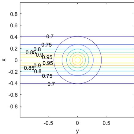
**Figure 1.** Contour plots on the ground of the coherence function for  $k_d = 0$  and for both cases of isotropic and extremely anisotropic fluctuations.  $f_c = 1$  GHz,  $L_0 = 10$  km,  $\sigma_N^2 = 0.1$
