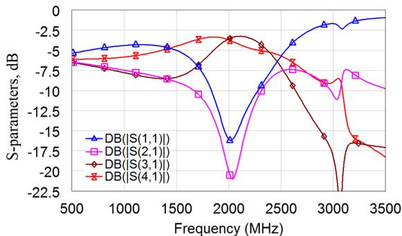
**Figure 8.** Measured frequency characteristics of a compact coupler.
