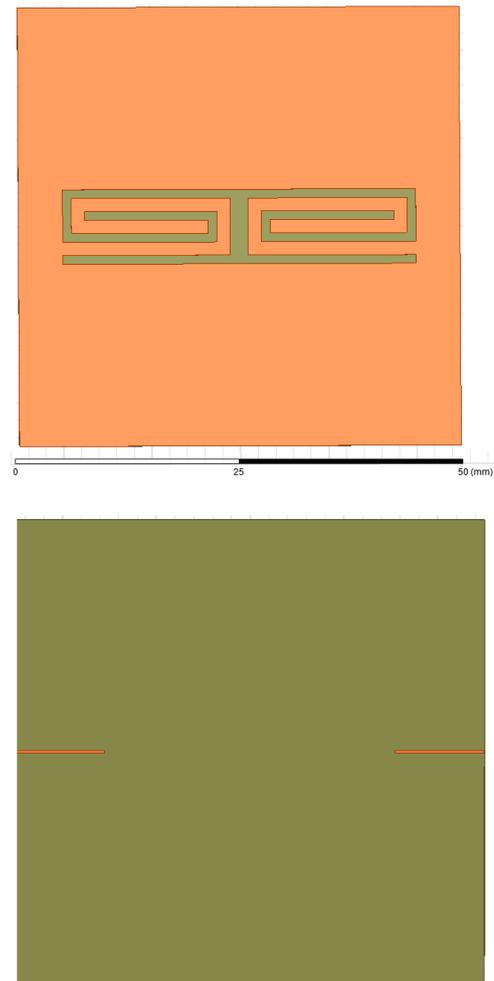
**Figure 1.** Top and bottom side of the bandpass filter.
