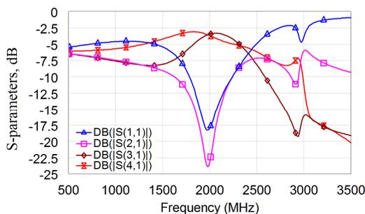
**Figure 4.** Frequency characteristics of a compact coupler.
