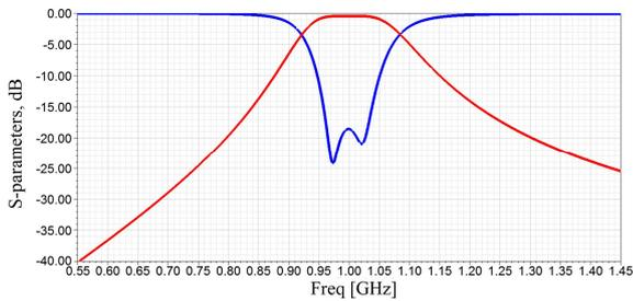
**Figure 2.** Frequency response of a bandpass filter.
