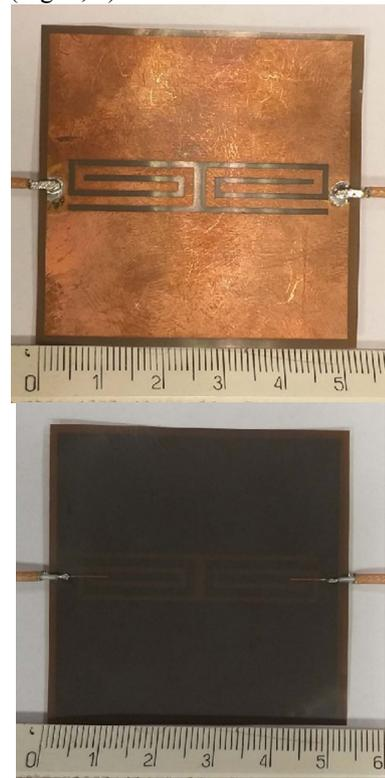
**Figure 5.** Top and bottom side of the bandpass filter.
