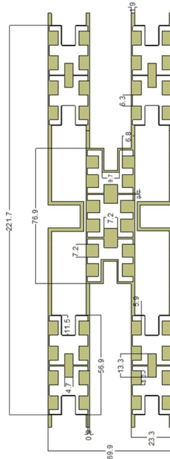
Figure 6. The layout of compact 4x4 Butler matrix for ATL.
