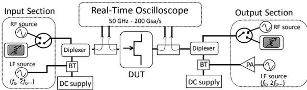
**Figure 1.** Low-frequency/high-frequency measurement setup implemented to perform the dynamic-bias characterization technique.
