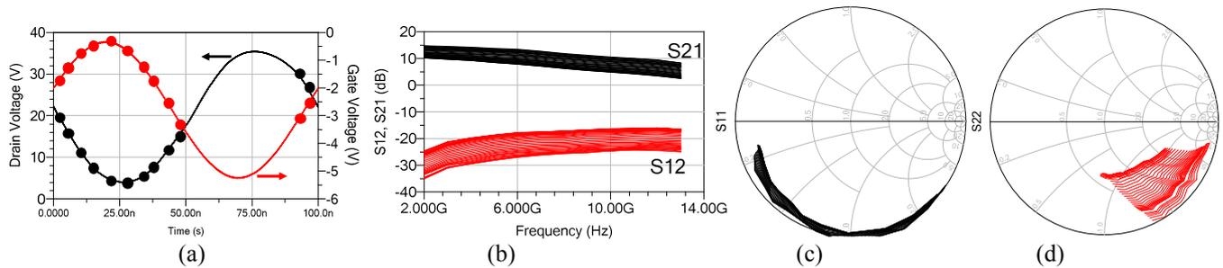
**Figure 5.** Multi-bias dynamic-bias S-parameters measurements performed on a 200- $\mu\text{m}$  GaN HEMT.  $f_{LF} = 10$  MHz.  $f_{HF}$  swept. (a) drain and gate voltages, (b)  $S_{21}$ ,  $S_{12}$  (c)  $S_{11}$  and (d)  $S_{22}$  parameters corresponding to the dots in (a).
