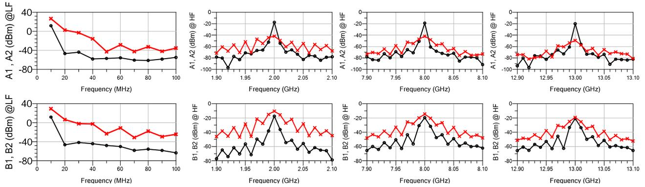
**Figure 3.** Spectra of incident (red crossed lines) and reflected (black circled lines) waves during dynamic-bias measurements performed on a 200- $\mu\text{m}$  GaN HEMT.  $f_{LF} = 10$  MHz.  $f_{HF}$  swept. High frequency spectra are reported for 2 GHz, 8 GHz and 13 GHz.
