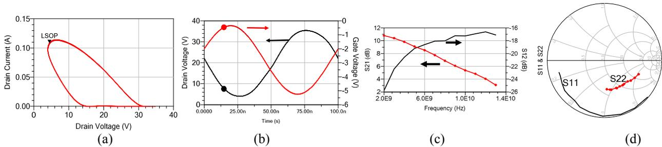
**Figure 4.** Dynamic-bias measurements performed on a 200  $\mu\text{m}$  GaN HEMT.  $f_{LF} = 10$  MHz.  $f_{HF}$  swept from 2 GHz to 13 GHz. (a) LSOP, (b) drain and gate voltages, (c)  $S_{21}$ ,  $S_{12}$  (d)  $S_{11}$  and  $S_{22}$  parameters corresponding to the dots in (b).
