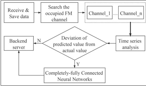
**Figure 2.** The flowchart of the FM broadcast monitoring system.
