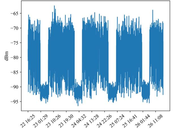
**Figure 4.** Time series data of four days for the FM channel 107.1MHz.
