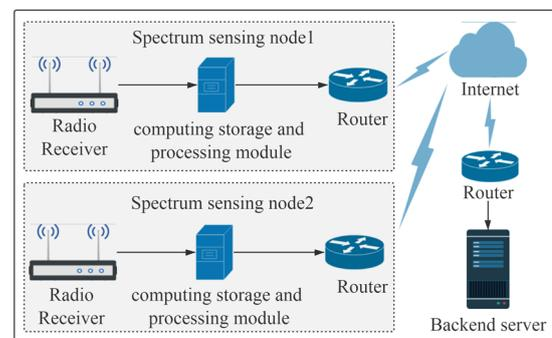
Figure 1 Architecture of the monitoring system.
