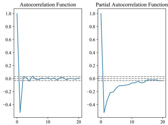
**Figure 5.** Estimating  $p$  and  $q$  parameters of ARIMA ( $p, d, q$ ) by ACF and PACF.
