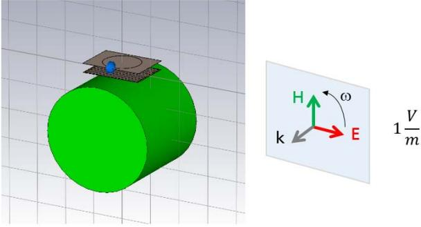
**Figure 2.** Full-wave model geometry and plane wave excitation depiction.
