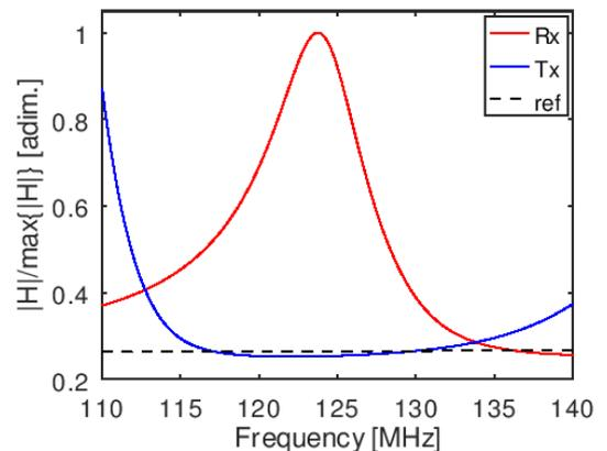
**Figure 3.** Normalized H-field magnitude at the phantom's surface for the Rx,  $C_v = 3.2$  pF (red), Tx,  $C_v = 4.7$  pF (blue), and the reference (dotted) case.
