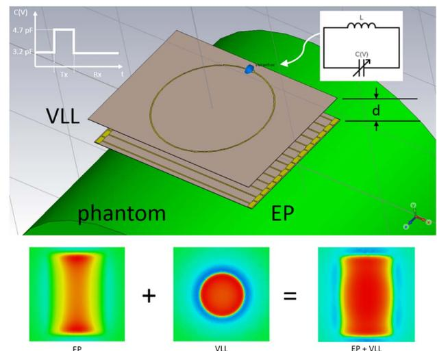
**Figure 1.** Sketch of the investigated Eigenmode problem. The DSEP is positioned 10 mm apart from a phantom (top). Illustration of the hybrid mode formation (bottom).
