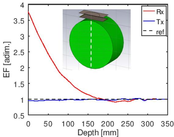
**Figure 4.** Simulation results for the field enhancement factor along the white dotted line in the inset at the operational frequency of 123.5 MHz.
