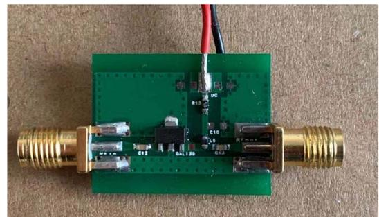
(a) The experiment board of the RF amplifier
