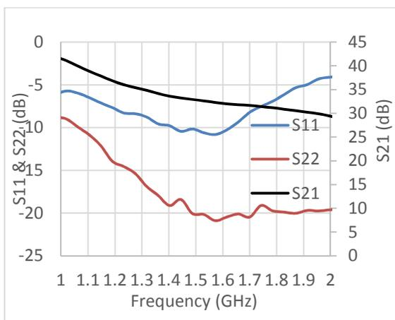
(b) S-parameter measurement results of the LNA
