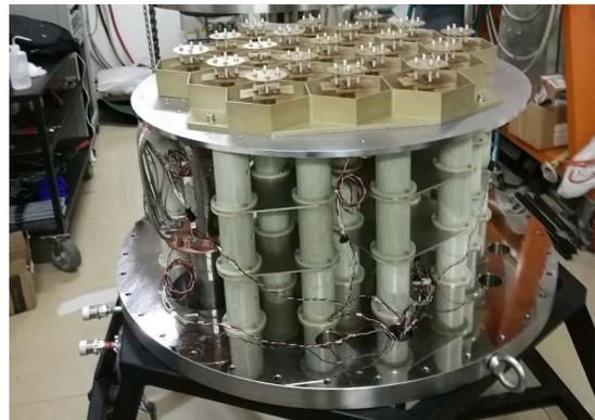
**Figure 1.** Cryogenic test on the antenna array of the 19-element PAF for FAST. The antenna array was installed in the cryostat supported by G10 pillars.
