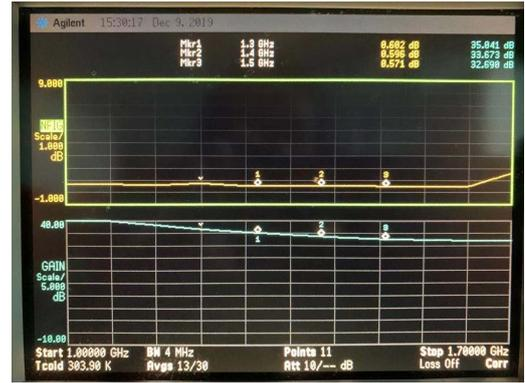
(c) The noise figure measurement of the LNA
