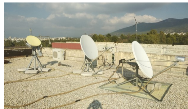
Fig 1. The NTUA beacon receivers (from left to right: Q-, Ku- and Ka-band)
