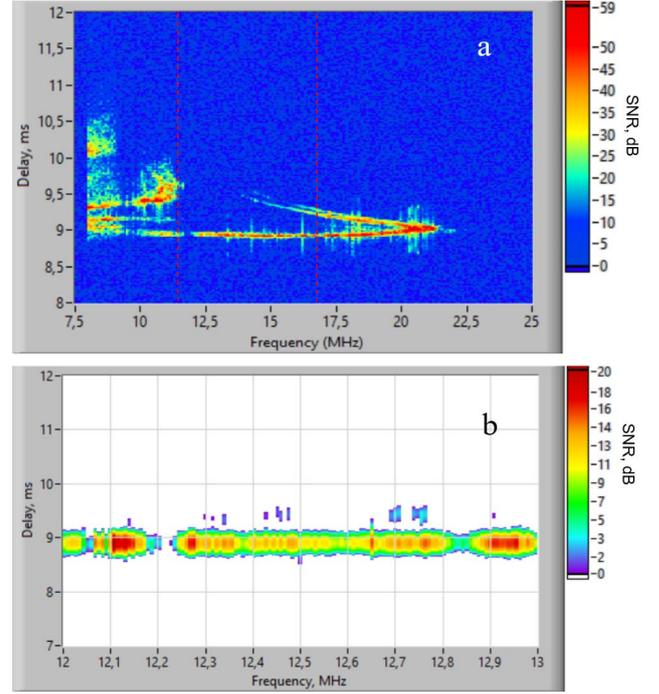
**Figure 2.** a) OIS ionogram of radio path of length 2.6 Mm recorded at 13/02/19 17:00 (LT) and SMPR; b) AFR of wideband (1 MHz) channel from SMPR.
