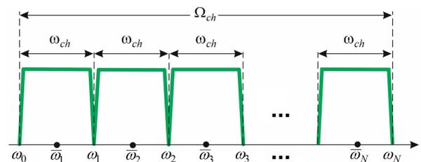
**Figure 1.** Partial narrowband channels that constitute the wideband channel.
