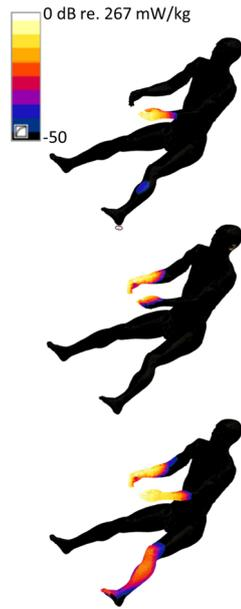
**Figure 3.** 3D representation of the distribution of the 10g average SAR induced on the skin of the phantom by the left antenna (top panel) and front antenna (mid panel) alone and by the four antennas simultaneously (bottom panel). Color map ranges from 0 to -50 dB (re: 267 mW/kg).
