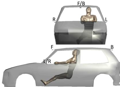
**Figure 1.** The exposure scenario. Frontal (top panel) and lateral view (bottom panel) of the realistic 3D model of the car, the human phantom and the four V2V antennas placed at the right (R), left (L), front (F), and back (B) sides of the car. Left and right antennas were placed near the car side mirrors. The dimensions of the car model are 3.8 (length) x 1.6 (width) x 1.3 m (height).
