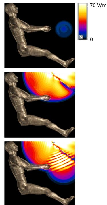
**Figure 2.** Distribution of the electric field E (rms value) generated by the left (top panel) and front antenna (mid panel) separately and by the four antennas simultaneously (bottom panel). E is evaluated on a sagittal plane at the midline of the phantom model. Color map ranges from 0 to 76 V/m (linear scale).
