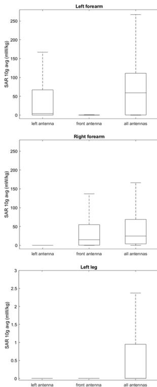
**Figure 4.** Boxplot of 10g average SAR induced in the skin of the left forearm (top panel), right forearm (bottom panel), and left leg (bottom panel) by the left and front antenna alone and by the four antennas simultaneously. Center lines in the boxes indicate the median; the bottom and top edges are the 25th and 75th percentiles. The whiskers correspond to approximately 99.3% of the values.
