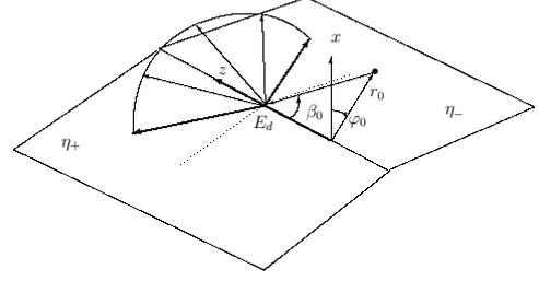
Figure 2: Edge wave and Keller's cone
