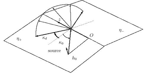
Figure 4: The edge wave excited by the primary surface wave
