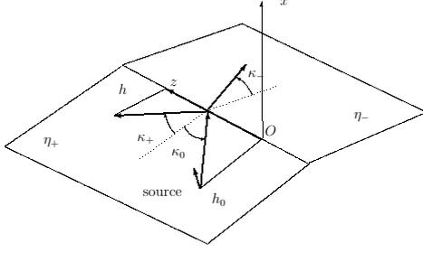
Figure 3: Reflected and transmitted surface waves by the edge
