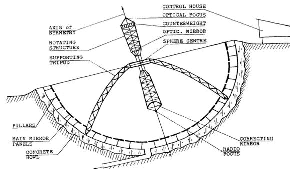
**Figure 1.** Arrangement of Radio-Optical Telescope ROT-54/2.6.
