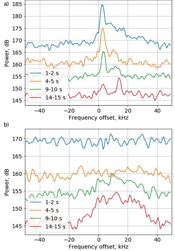
**Figure 4.** The dynamics of the development of the downshifted plasma line spectra during prolonged quasi-continuous heating for different exposure times (time shift  $\sim 5$  s) at two fixed heights  $h_1 = 214$  km (panel a)) and  $h_2 = 210.8$  km (panel b)). Averaging over 50-55 PW pulses was performed out. An additional shift of each spectra by 5 dB was used. 11/08/2018, 17:46:00-17:46:15 LT.
