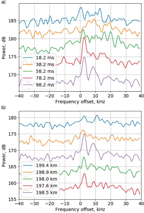
**Figure 3.** The dynamics of the downshifted plasma line spectra at the stage of Langmuir turbulence development for different pumping times with a step of 20 ms at a fixed height  $h = 198.5$  km (panel a)) and the altitude distribution with a step of 450 m of spectral intensity towards the end of the PW pulse  $t = 98.2$  ms (panel b)). Averaging over 50-55 PW pulses was carried out. An additional shift of each of the spectra by 5 dB was used. 11/08/2018, 15:51:30-16:11:30 LT.
