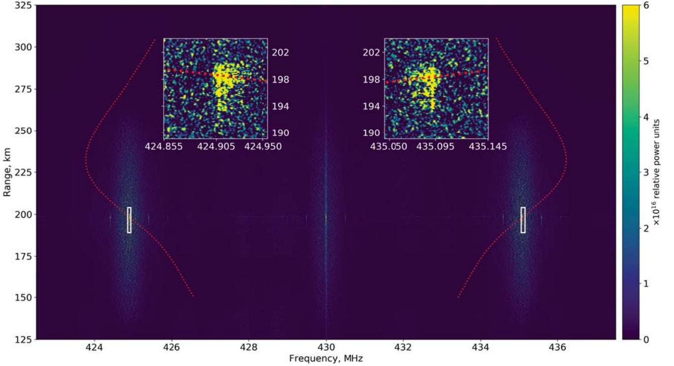
**Figure 2.** Electron density profile and spectrogram of artificial ion and plasma lines (downshifted plasma line on the left, upshifted plasma line on the right for 98.2 ms of pumping). Separate panels show the region of generation of the plasma line with a high frequency-altitude resolution. 11/08/2018, 15:51:00-16:11:30 LT.
