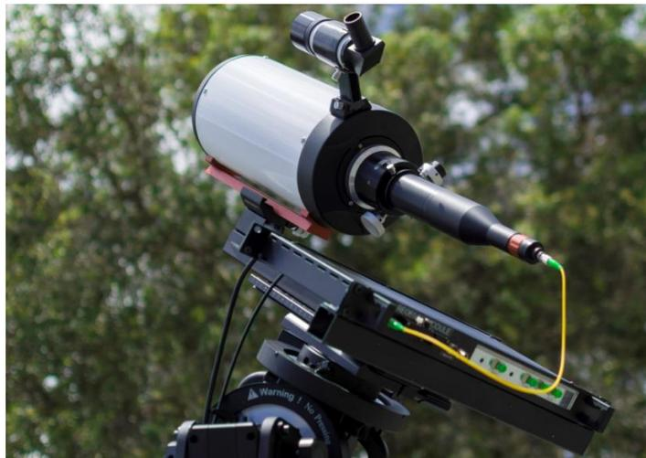
**Figure 1.** Optical terminal for the free-space phase-stabilized frequency transfer system.
