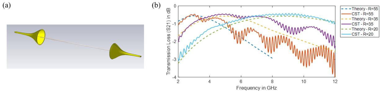
**Figure 1.** (a) SW transmission line, (b) Transmission loss results for the SW transmission line.
