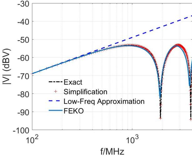
**Figure 2.** Coupled voltage (in dBV) to load of a straight trace with change in operating frequency. Other input parameters are : trace length ( $L$ ) = 85.6 mm, trace width ( $W_s$ ) = 3.81752 mm, dielectric thickness ( $h$ ) = 2 mm,  $\epsilon_r = 4.4$ ,  $\tan \delta = 0.02$ ,  $\theta = \phi = \gamma = 0^\circ$ .
