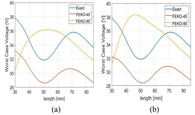
**Figure 3.** Worst-case coupled voltage vs length of the trace for three different trace shapes at (a) Load 1 and (b) Load 2.
