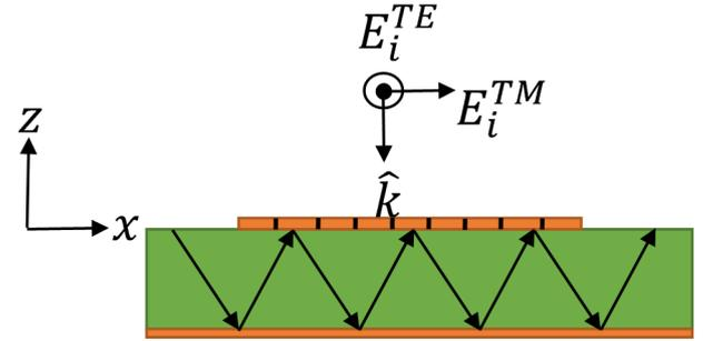
**Figure 1.** A conductive trace (top orange) located above dielectric (green) backed by ground plane (bottom orange).
