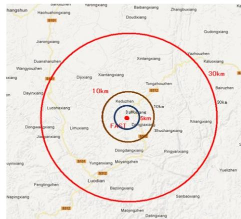
**Figure 1.** Distribution of FAST RQZ: the core zone with the radius of 5 km, the middle zone with the radius between 5 and 10 km, and the remote zone with the radius between 10 and 30 km.
