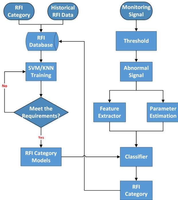
**Figure 2.** Flow chart of the RFI intelligent identification system.
