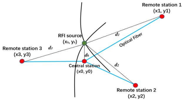
**Figure 3.** Schematic illustration of TDOA algorithm.
