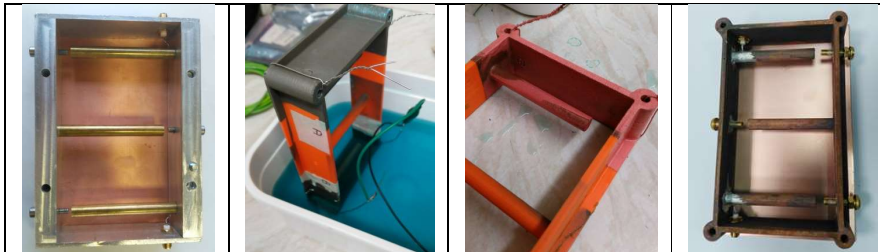
Figure 1. Three-pole interdigital band-pass filter and 3D printed variant during stages of electroplating.
