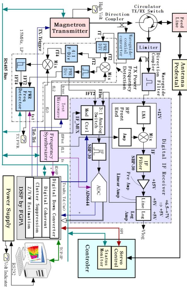
**Figure 3.** WXR-MD-10 Block Diagram (Note that the DDC-Digital Down Converter in Digital IF Receiver is put on DSP-Digital Signal Processor).
