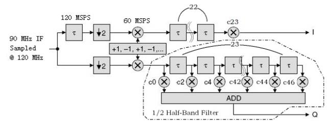
**Figure 4.** The orthogonal processing of DDC in FPGA.
