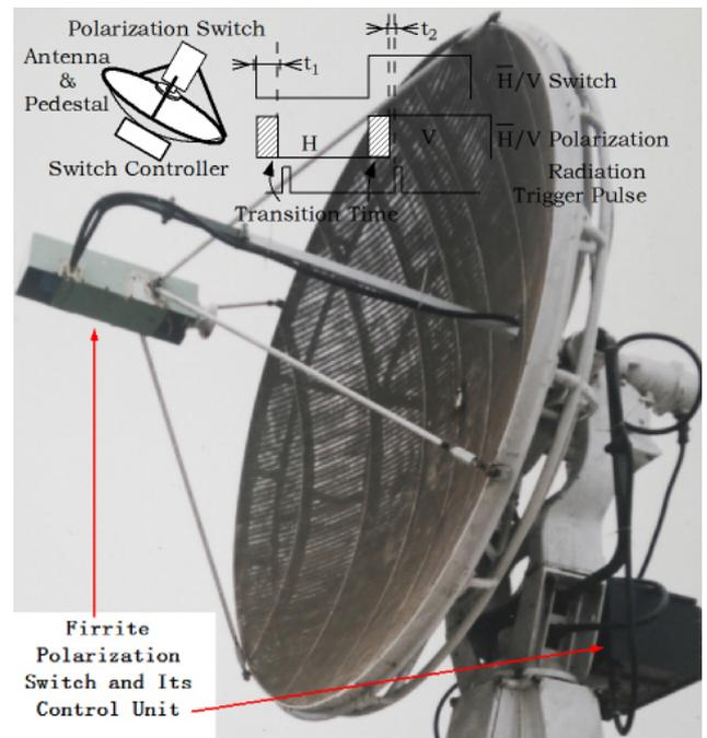
**Figure 2.** Dual-polarization Antenna with Polarization Switch and Controller for XDPR Radar System.
