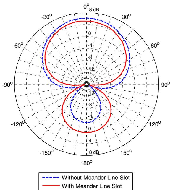
**Figure 3.** Comparison of Radiation Pattern
