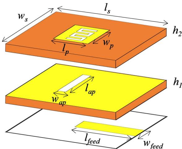
**Figure 1.** Aperture Coupled Microstrip Antenna with Meandered Slot
