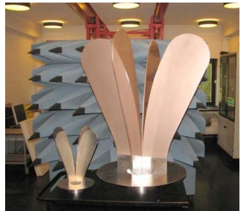
**Figure 3: 1-3GHz and 0.4-1.2GHz dual-port quad-ridge probes.**
