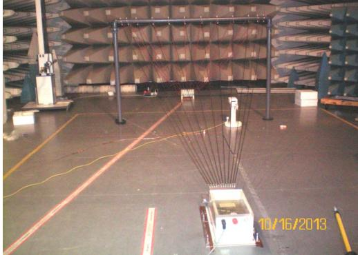
Fig. 1 The conical EMP simulator in BIRMM lab
