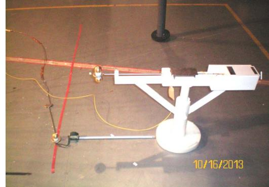
Fig. 2 The designed probe fixture
