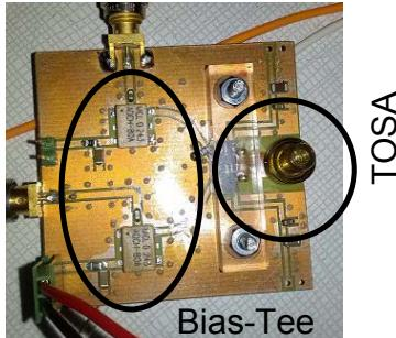
**Figure 2. VCSEL test bench**
