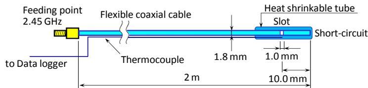
Fig. 2 Basic structure of coaxial-slot antenna.
