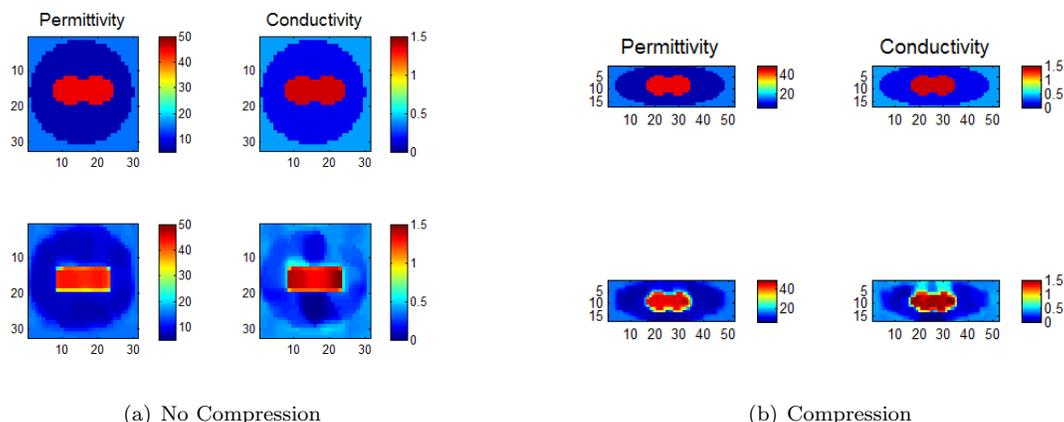
Figure 2: Reconstruction results for the object with and without compression after 3000 iteration steps. The permittivity (columns 1 and 3) and conductivity (columns 2 and 4) of the original (top) and reconstructed object (bottom). The axes are indexed by pixel number.
