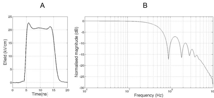
Fig. 1: A - Example of a typical pulse applied during cloning efficiency experiments. The measurement was made using a D-dot sensor. Integration of the signal from the D-dot was made numerically with Matlab. B –Normalized frequency content of the pulse.
