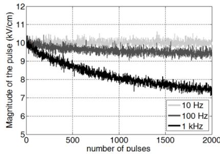
Fig. 4: Evolution of the pulse magnitude due to temperature increase when a high number of pulses are applied.
