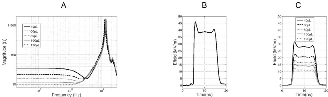
Fig. 2 : A- Impedance of cuvettes containing different volumes of SMEM. B –Measurement of the pulse applied on an adapted load. C- Measurements of the resulting pulses applied on the cuvettes for different volumes of medium.
