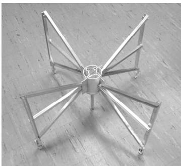
Figure 3. MWA antenna without LNAs
