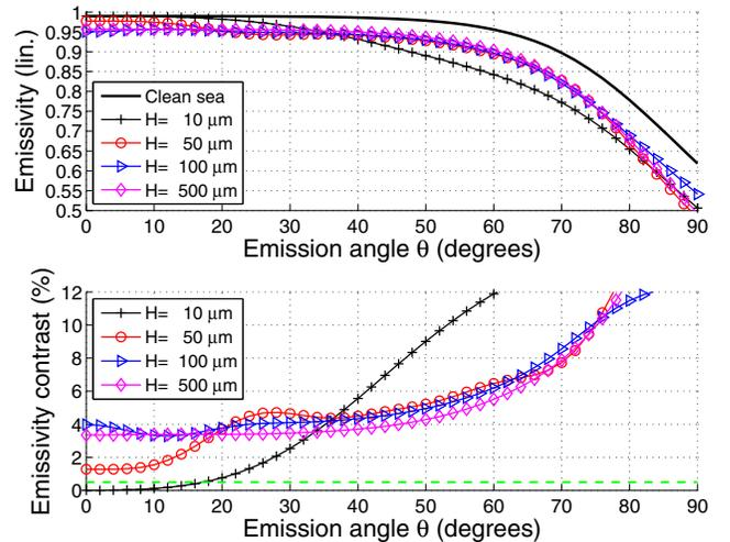
**Fig. 2.** Unpolarized emissivity (upper sub-figure) of clean and contaminated seas and emissivity contrast of contaminated seas with respect to clean seas (lower sub-figure) versus the emission angle  $\theta$  for a wavelength  $\lambda = 10$   $\mu$ m and for wind speed  $u_{10} = 5$  m/s and direction  $\phi = 0$ . For the contaminated sea, the oil viscosity  $\nu_{oil} = 0.5$  cm<sup>2</sup>/s, and the oil film thickness  $H = \{10, 50, 100, 500\}$   $\mu$ m.
