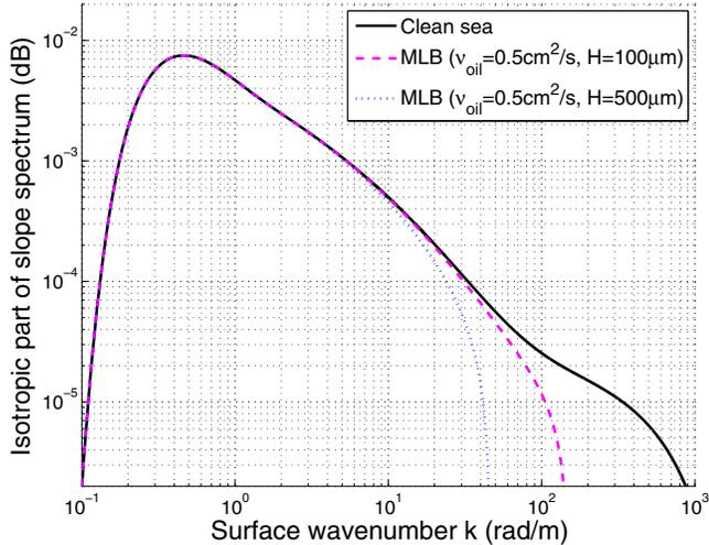
**Fig. 1.** Isotropic part of the surface slope spectrum of clean and contaminated seas versus the surface wavenumber  $k$ , for a wind speed  $u_{10} = 5$  m/s. For the contaminated sea, the oil viscosity  $\nu_{oil} = 0.5$  cm<sup>2</sup>/s, and the oil film thickness  $H = \{100, 500\}$   $\mu$ m
