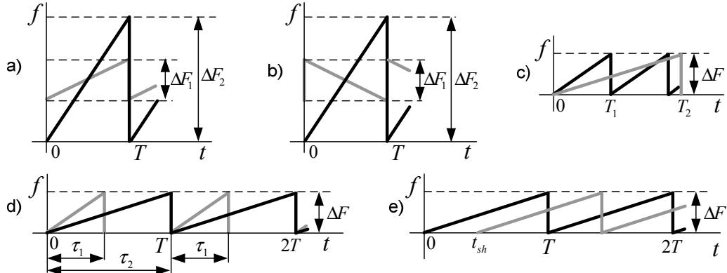
Figure 1: Some degrees of freedom for the LFM signals' generation.
