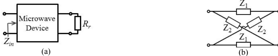
Fig. 1. Reactive network terminated in a single resistance (a) and equivalent bridge circuit of a symmetric reciprocal two-port (b).
