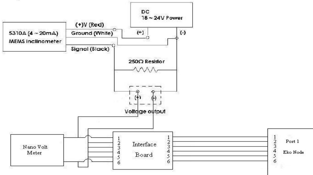
Fig. 2 Digital Sensor Connection with Eko system
