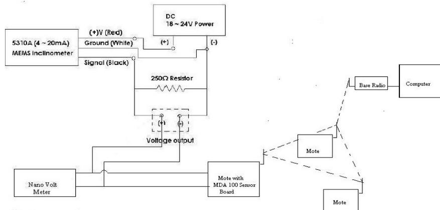
Fig.1 Digital Sensor Connection with IRIS Mote
