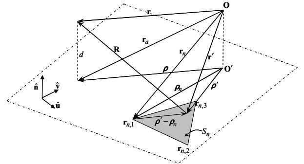
Figure 2. Vector definitions for a triangular patch.
