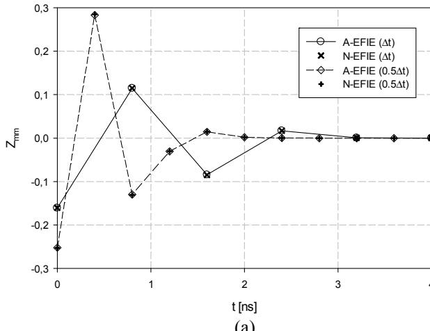
Figure 3. MOT matrix elements of EFIE for different time step sizes.
