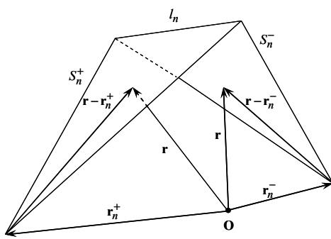
Figure 1. Definition of the RWG basis.
