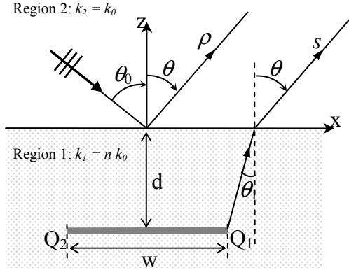
Fig. 1 – Geometry for the scattering by a buried strip.
