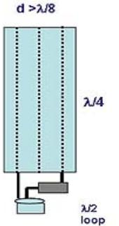
Figure 6. MB antenna feeding points.
