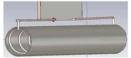
Figure 8. Coil delay line.
