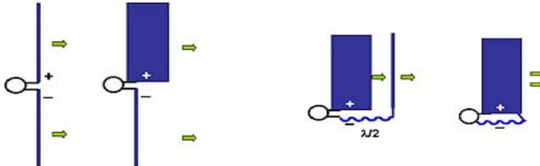
Figure 4. First stage of the MB antenna design.
