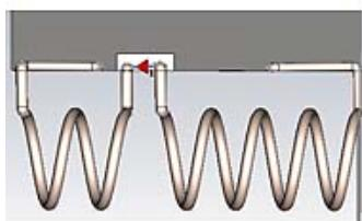
Figure 13. Delay line construction for the 2GHz band.
