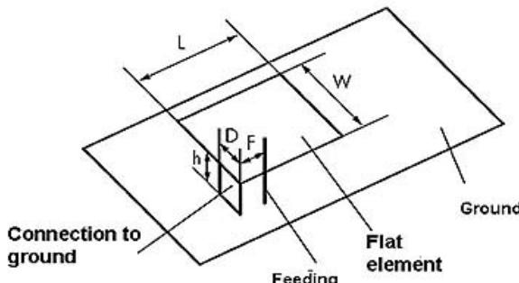
Figure 2 Principal construction of PIFA
