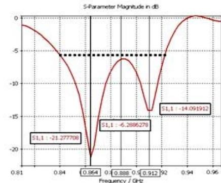
Figure 12. S11 of MB with a doubled bandwidth.
