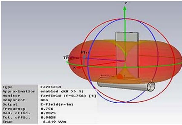
Figure 9. MB antenna radiation patterns in far field
