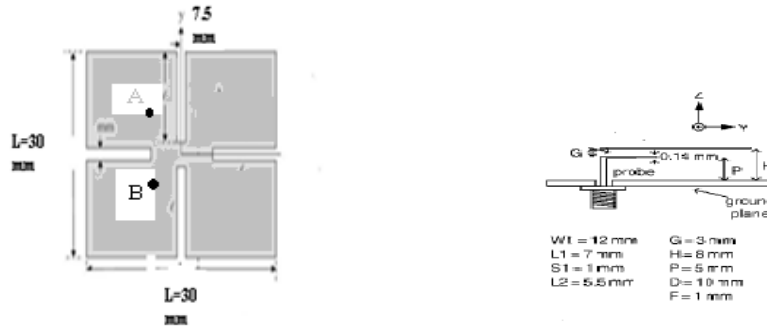
Fig. 1 Geometry of proposed square-fed flower -shaped Microstrip patch antenna
